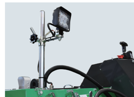
▲作業灯(LED)増設
